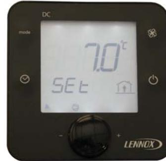
This is a remote controller for non-technical customer. It is designed to fit aesthetically inside a room and be very easy to use. It has a 24V supply to be connected to the unit and can be installed at maximum 30 meters away from the unit.
