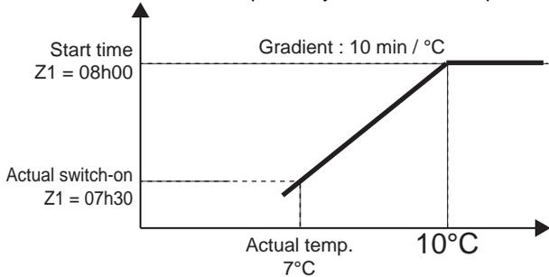
of the most difficult applications in terms of occupation and varying internal loads, the new eCLIMATIC offers now up to 7 time zones per day (Z0 to Z6) adjustable by steps of 10 minutes. Each time zone can be programmed to follow one of four possible operating modes:
