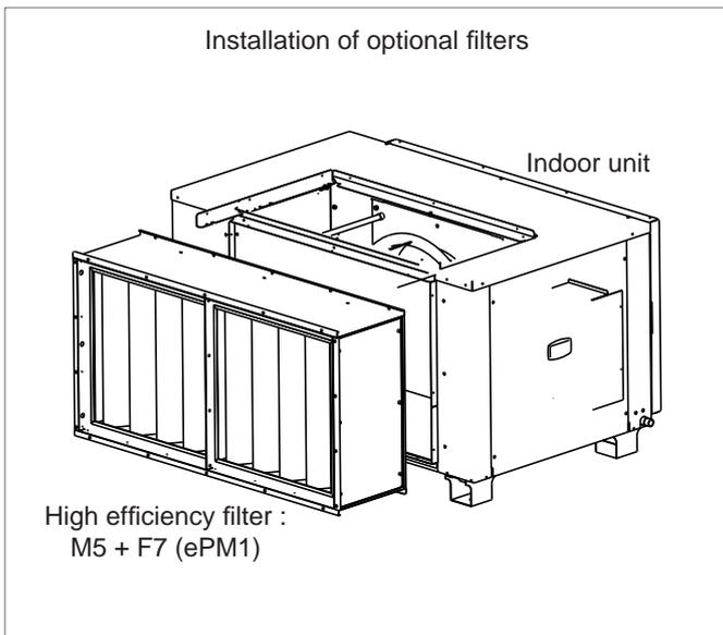
As standard, the unit are delivered with G4 filters.
