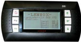
This plug and play service display and controller allows service personal to set up to read and modify all unit parameters (Unit settings, operating time and number of compressor starts, low and high pressure reading, airflow rate of supply fan, and read the history of last 32 faults...).
