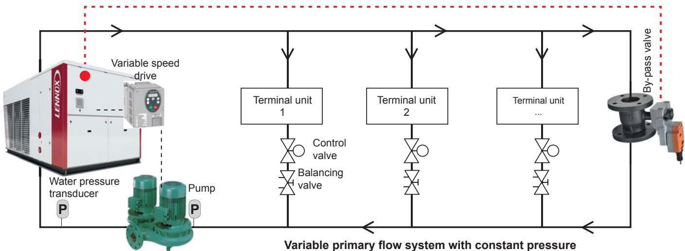
A variable primary flow design uses fewer components than primary–secondary systems as the pumps of the secondary distribution loop and the mixing tank are eliminated.
