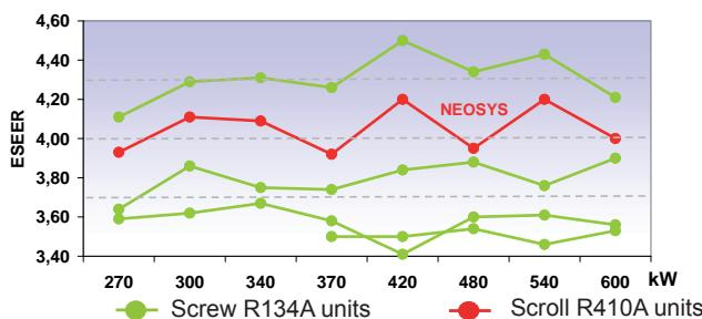
By using R410A refrigerant associated with high efficiency micro channel coils and variable speed fans NEOSYS is contributing to a very low energy consumption all year around with an average energy efficiency ratio (ESEEER)\* in cooling mode above 4.0. NEOSYS Heat-pumps are also achieving very high performances in cooling and heating mode (COP\* up to 3.2).
