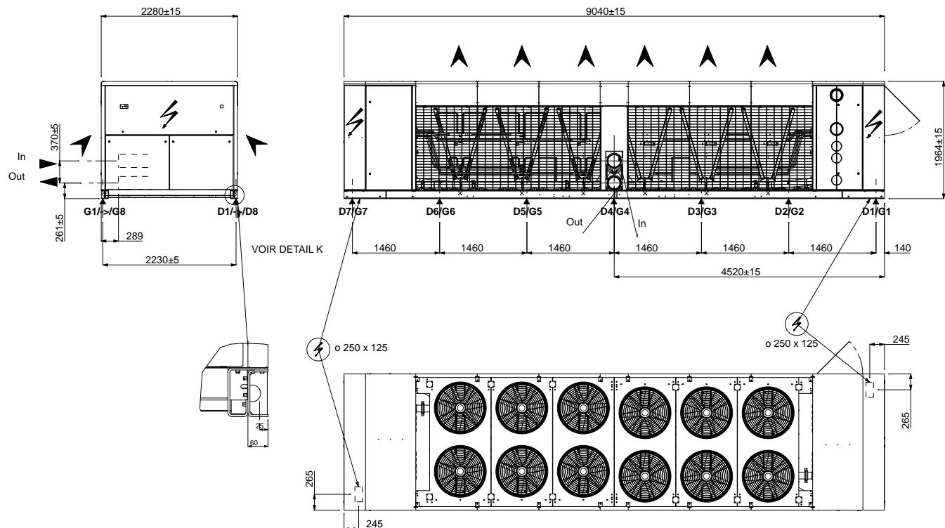
**LEGENDE:****IN** Water inlet**OUT:** Water outlet
